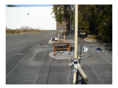
**Radiated Emission - Rear View with Trucker Antenna**
