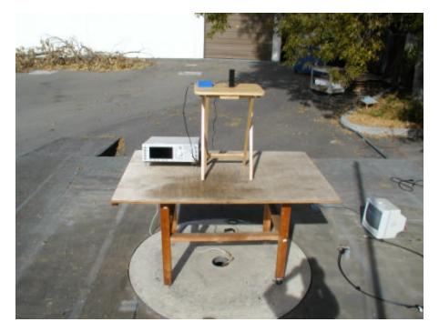
**Radiated Emission - Rear View with Stealth Antenna**
