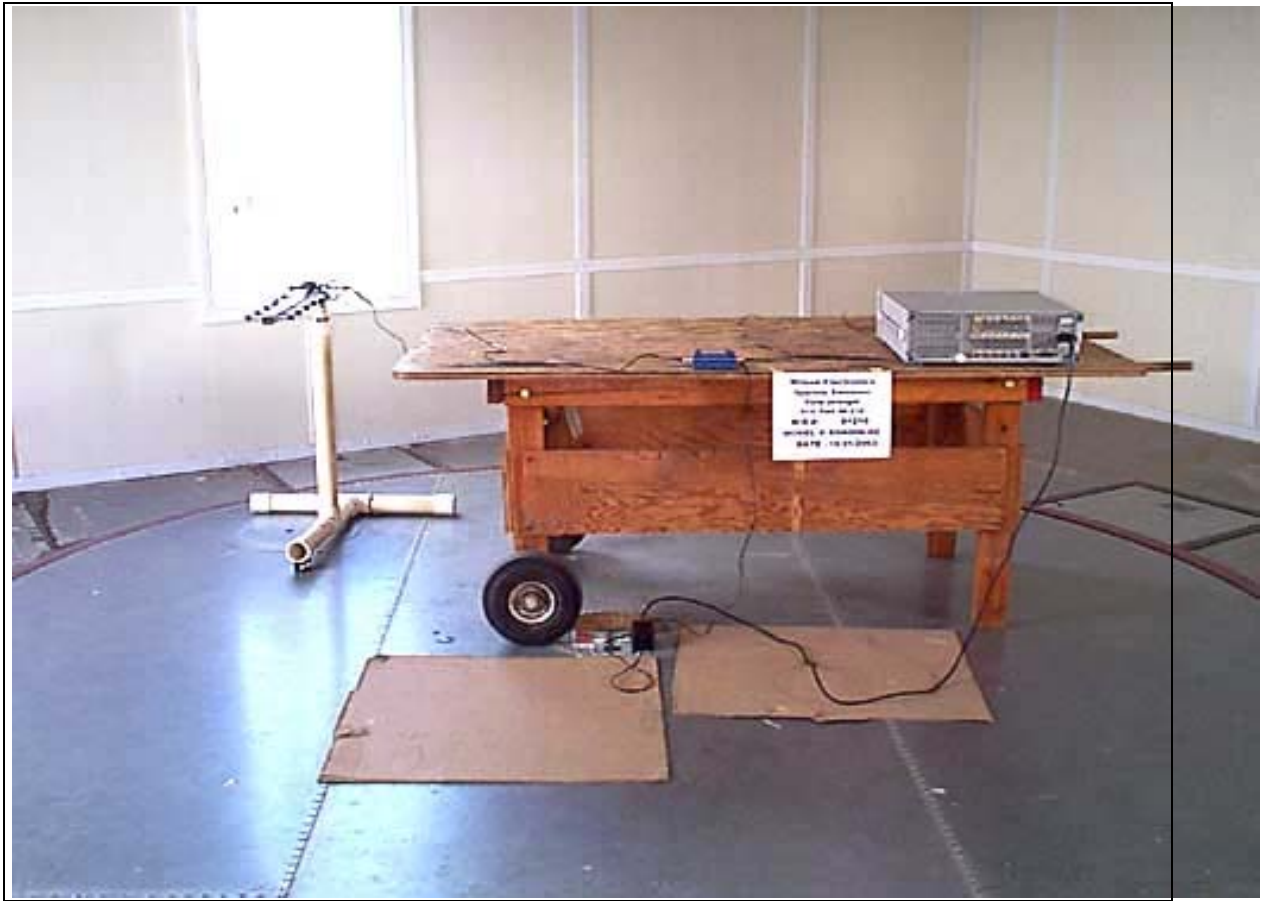
Radiated Emissions - Back View Downlink Side - Yagi Antenna
