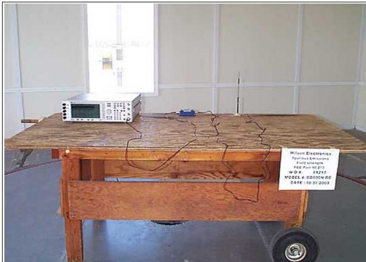
Radiated Emissions - Front View Downlink Side - Whip Antenna
