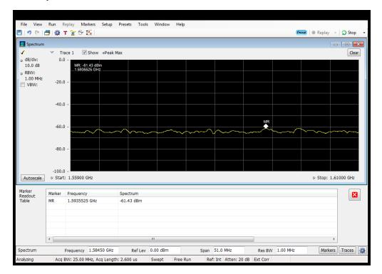
Conducted Spurious Emission\_UL\_776 - 787 MHz\_measured 1559 - 1610 MHz\_RBW 1 MHz
