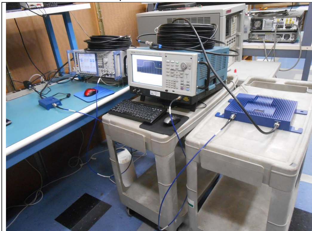
RF Conducted #1 Main unit, InLine unit and 300 Foot Cable
