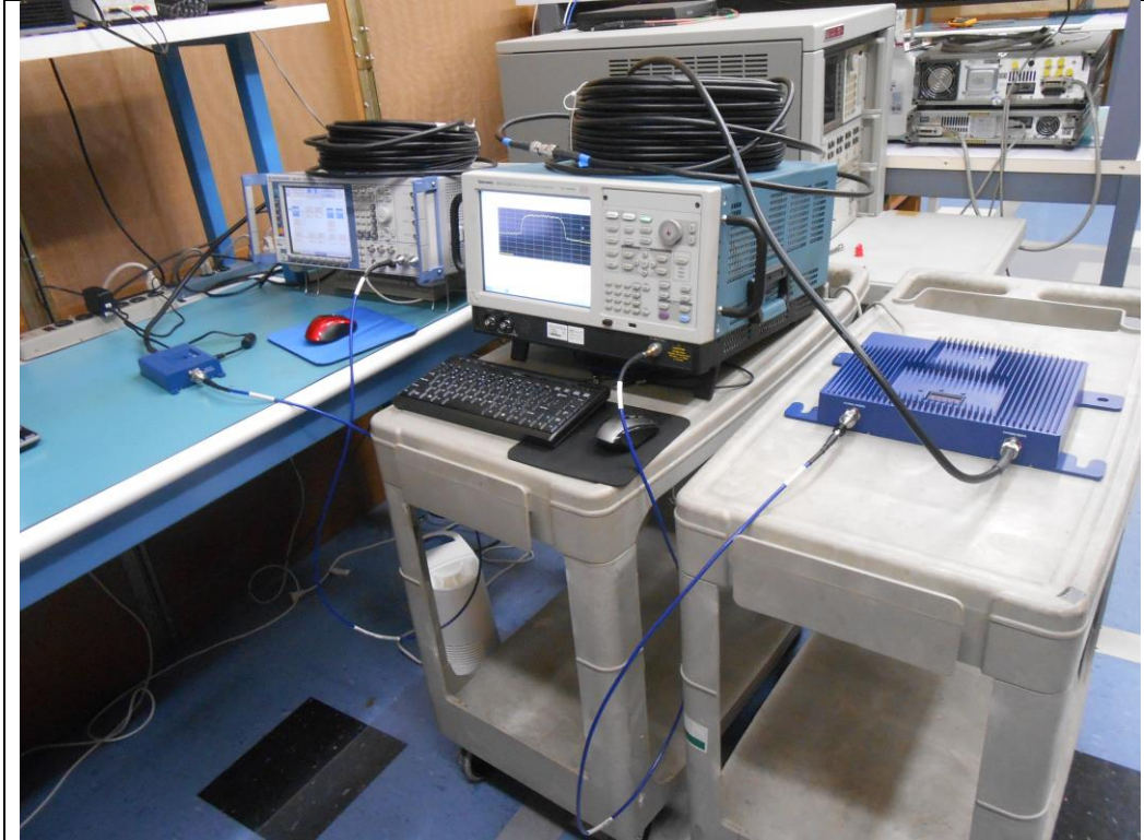
RF Conducted #1 Main unit, InLine unit and 300 ft cable
