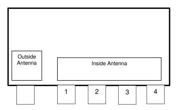
For all tests, the unused server ports (any port not being tested) was terminated with 50 ohm termination.
