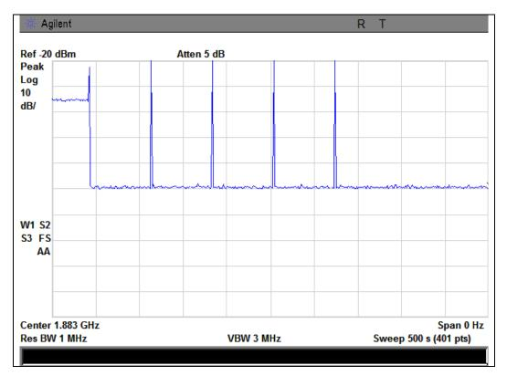
Downlink Detection Time Test Results 728 - 746 MHz Band
