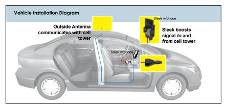
NOTE: The cell phone must be placed in the cradle to work properly.
