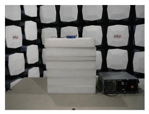
10.2 Radiated Emissions 30 MHz to 1 GHz- Rear View
