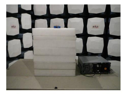
13.2 Radiated Emissions 30 MHz to 1 GHz- Rear View
