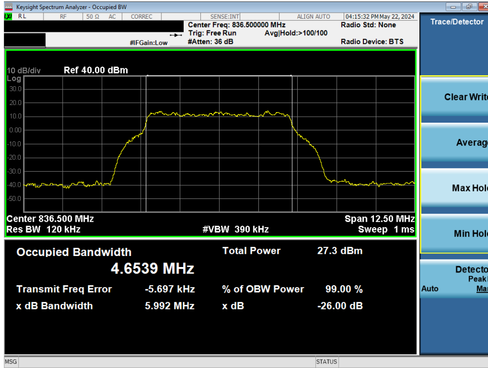
Plot 7-218. Occupied Bandwidth – BAND 5 UL QPSK (Output)
