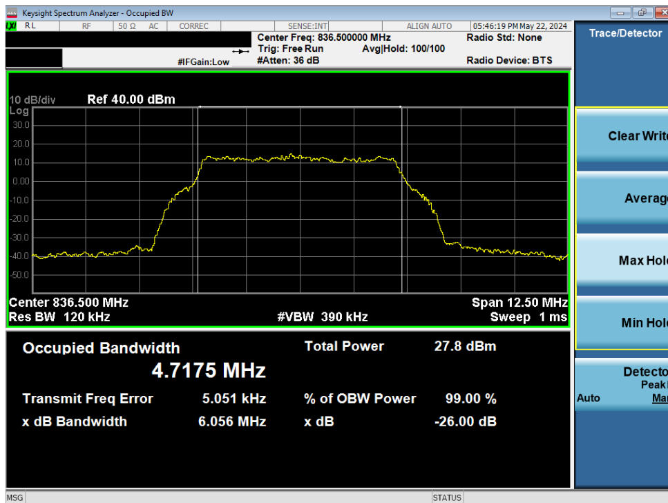
Plot 7-219. Occupied Bandwidth – BAND 5 UL 256-QAM (Output)
