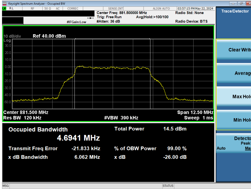
Plot 7-214. Occupied Bandwidth – BAND 5 DL QPSK (Output)
