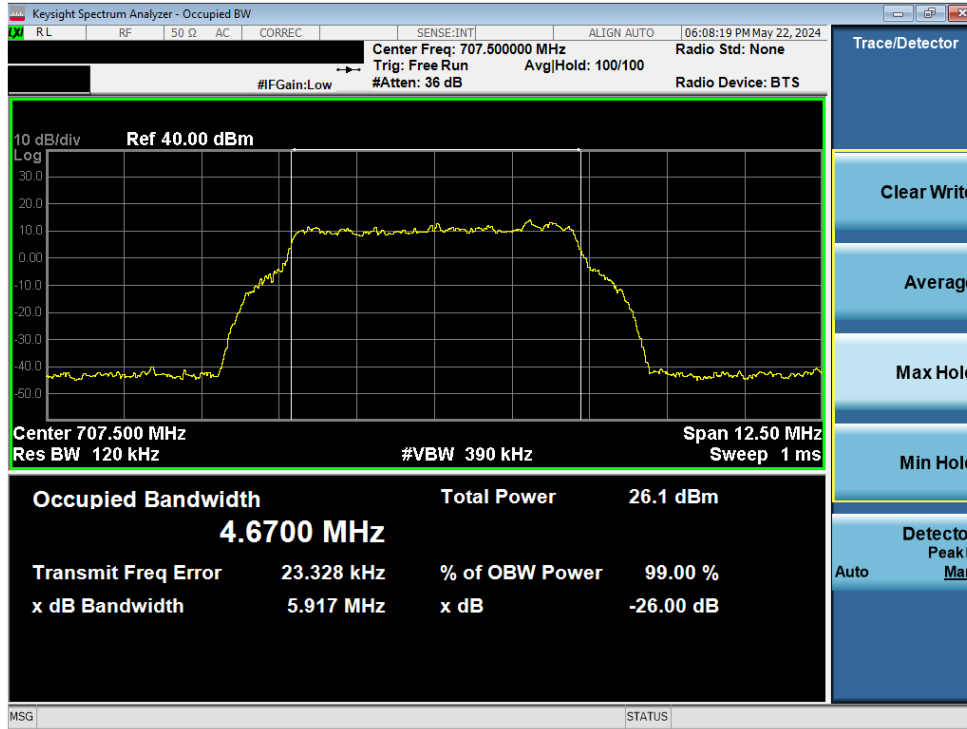
Plot 7-226. Occupied Bandwidth – BAND 12 UL QPSK (Output)
