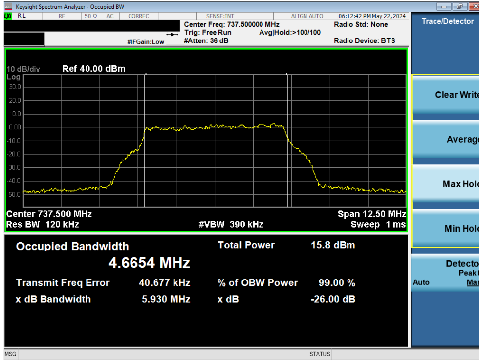
Plot 7-222. Occupied Bandwidth – BAND 12 DL QPSK (Output)
