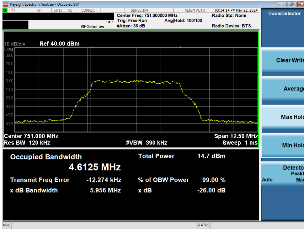
Plot 7-230. Occupied Bandwidth – BAND 13 DL QPSK (Output)
