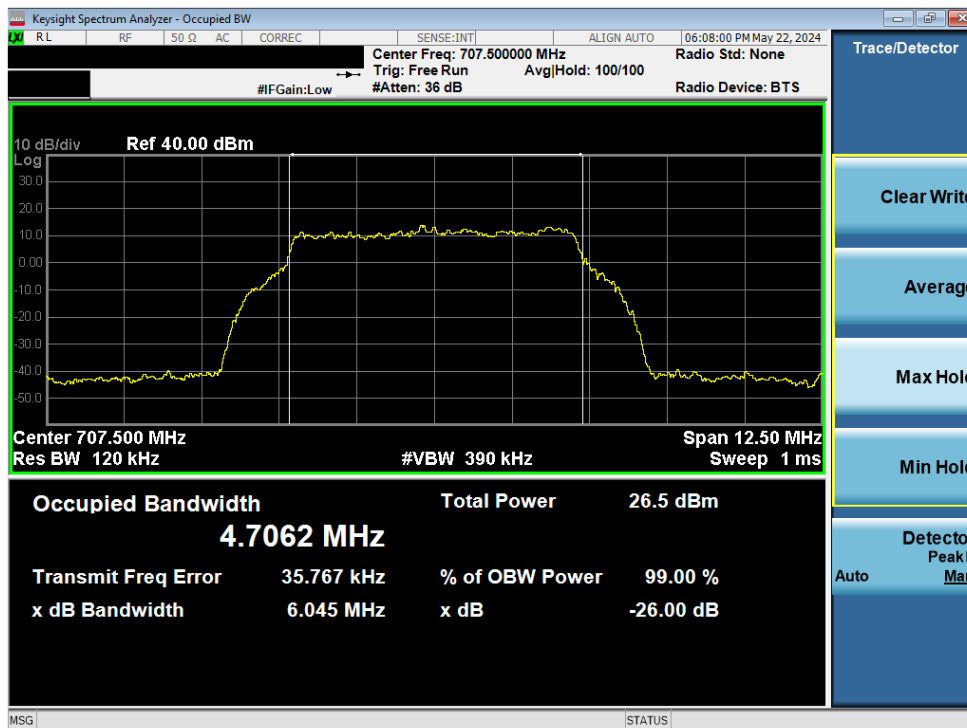
Plot 7-227. Occupied Bandwidth – BAND 12 UL 256-QAM (Output)
