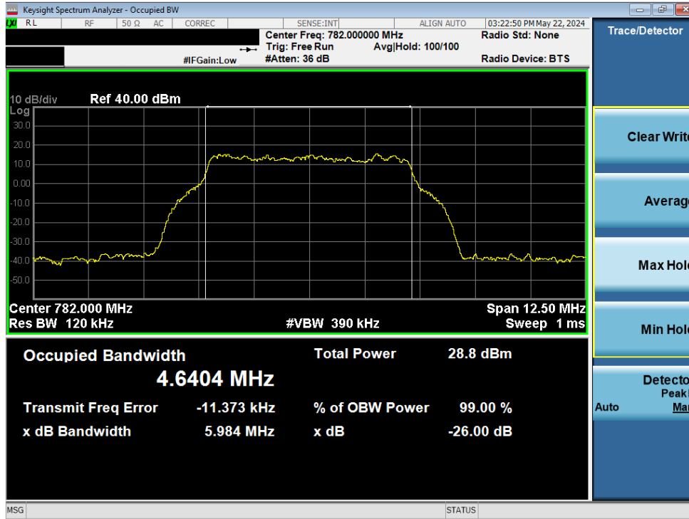
Plot 7-234. Occupied Bandwidth – BAND 13 UL QPSK (Output)
