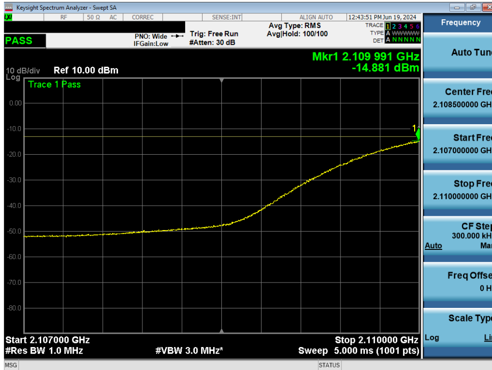
Plot 7-92. Out of Band Emissions – Band 4 DL Lower OOB @ 10dB above AGC
