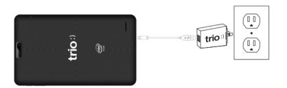
Plug the charger into a power outlet. The screen will display a flashing battery symbol for a few seconds to show that the battery is charging. Keep the battery on charge for 6 to 8 hours to make sure that it is fully charged.
