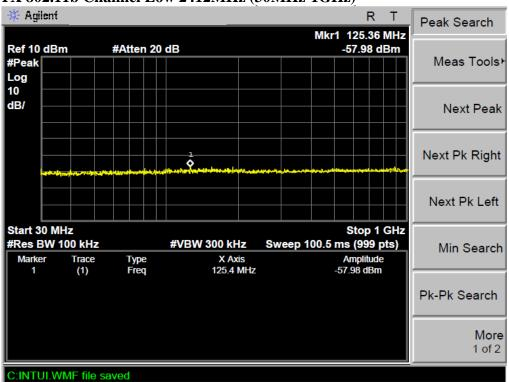
TX 802.11b Channel Low 2412MHz (1GHz-25GHz)
