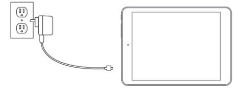
Plug the charger into a power outlet. Keep the battery on charge for 6 to 8 hours to make sure that it is fully charged.
