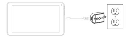
Plug the charger into a power outlet. The screen will display a flashing battery symbol for a few seconds to show that the battery is charging. Keep the battery on charge for 6 to 8 hours to make sure that it is fully charged.
