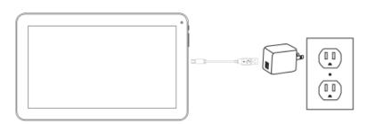
Plug the charger into a power outlet. The screen will display a flashing battery symbol for a few seconds to show that the battery is charging. Keep the battery on charge for 6 to 8 hours to make sure that it is fully charged.
