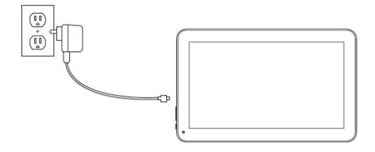
Plug the charger into a power outlet. The screen will display a flashing battery symbol for a few seconds to show that the battery is charging. Keep the battery on charge for 6 to 8 hours to make sure that it is fully charged.
