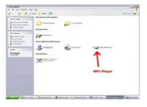
4.Locate the drive created by the unit, generally just called Removable Disk, with a letter in Parenthesis. Drive letters vary depending on your system configuration.
