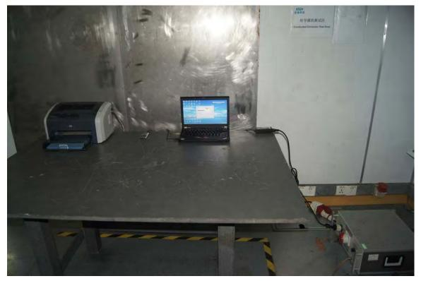
Radiated emissions test 30MHz- 1GHz Transfer data & Charging
