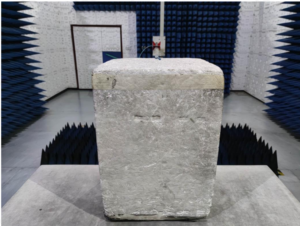
RADIATED EMISSION TEST SETUP ABOVE 1GHZ
