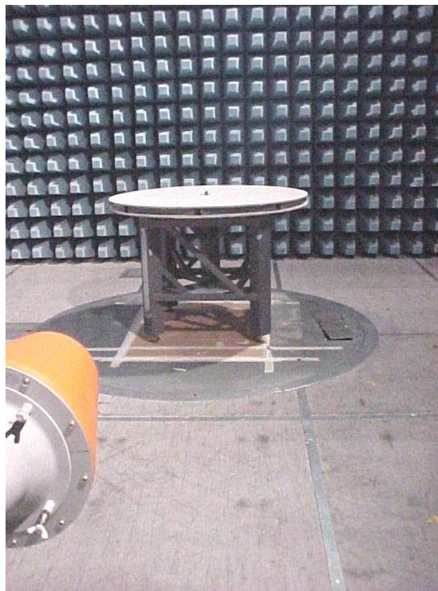
PHOTO N° 2 – SET-UP FOR EMISSION RADIATED TEST
