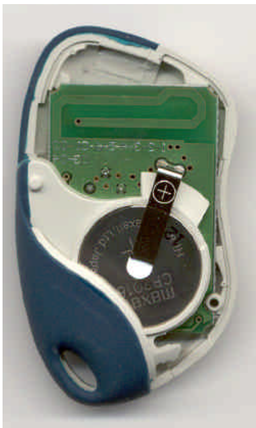
TX SETW295AM2 – Back internal view
