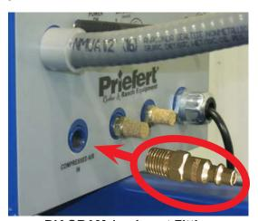
**DIAGRAM 1 - Insert Fitting** (Male, 1/4" NPT Quick-Connect Shown)
