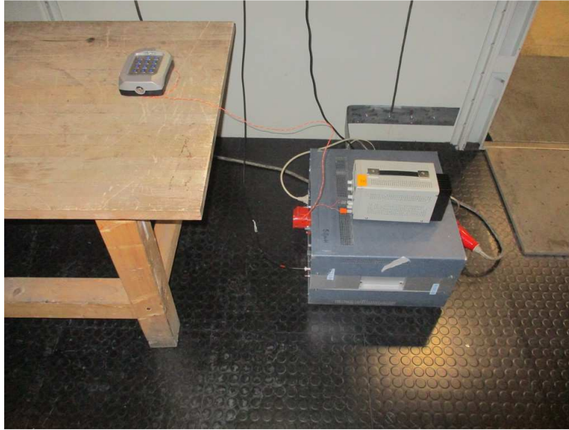
Conducted emission set-up 150kHz – 30MHz
