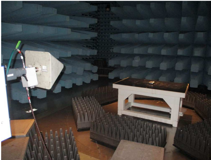
Radiated emission set-up above 1 GHz
