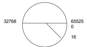
Once the serial number of the transmitter has been stored into the receiver memory, is the counter number received and the counter number of the receiver differ for less of 16, the receiver updates its counter and enable the output.
