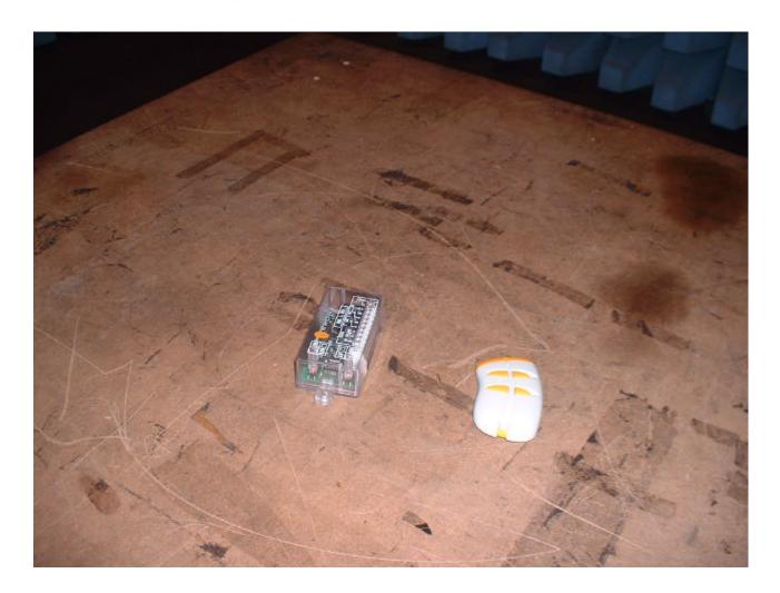
6.0.1 – Radio interference field strength radiated
