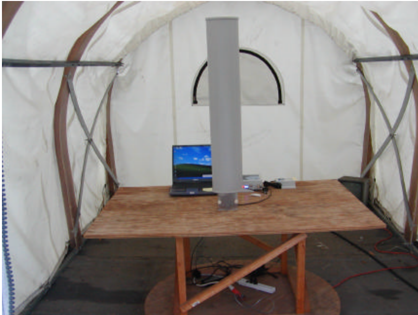
Radiated Emission – EUT with PAWSA24-16 16.5dBi Vertically Polarized 120 Degree Sector Antenna Front View
