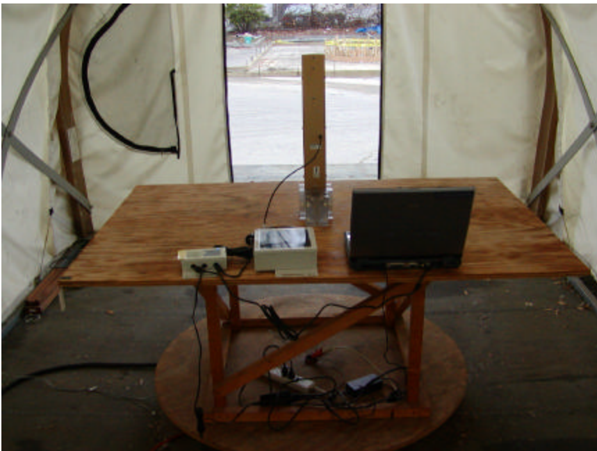
Radiated Emission – EUT with WISP 24013-90PTNF 14dBi 90 Degree, Sector Panel Antenna Rear View
