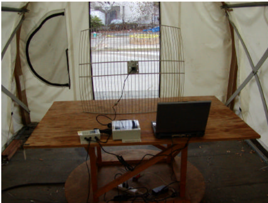
Radiated Emission – EUT with WISP 24024 PTNF 24dBi parabolic Grid Antenna Rear View
