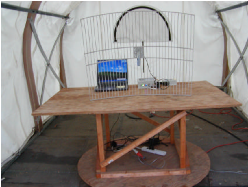
Radiated Emission – EUT with WISP 24024 PTNF 24dBi parabolic Grid Antenna Front View
