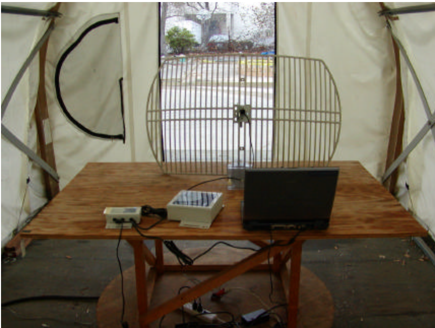
Radiated Emission – EUT with PAWDC24-HD-PFIP 24dBi Die Cast Antenna Rear View
