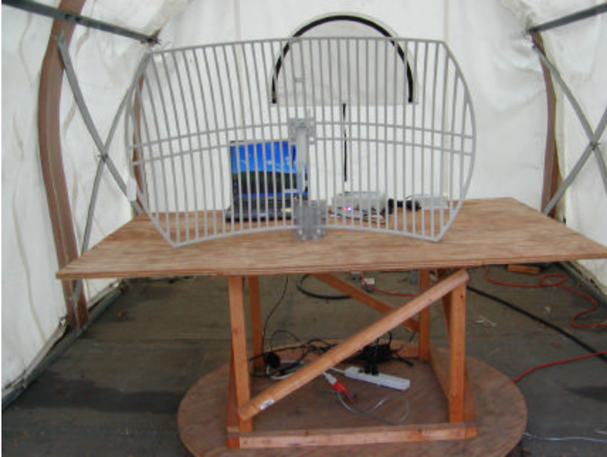
Radiated Emission – EUT with PAWDC24-HD-PFIP 24dBi Die Cast Antenna Front View
