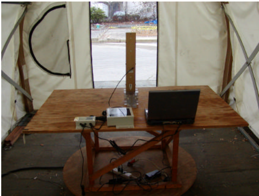
Radiated Emission - EUT with WISP 24013-120PTNF 13dBi 120 Degree, Sector Panel Antenna Rear View
