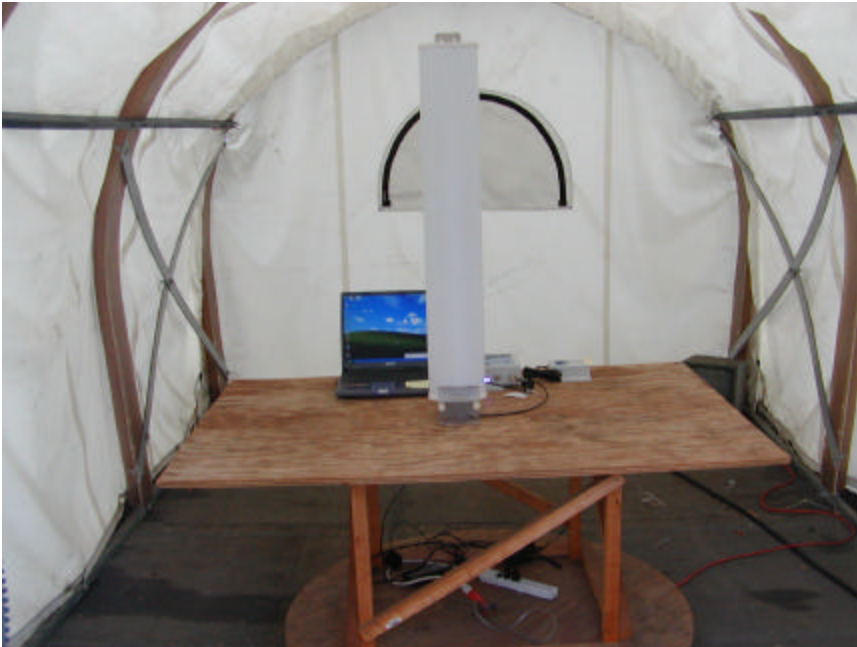
Radiated Emission – EUT with PAWSA24-17 17dBi Vertically Polarized 90 Degree Sector Antenna Front View
