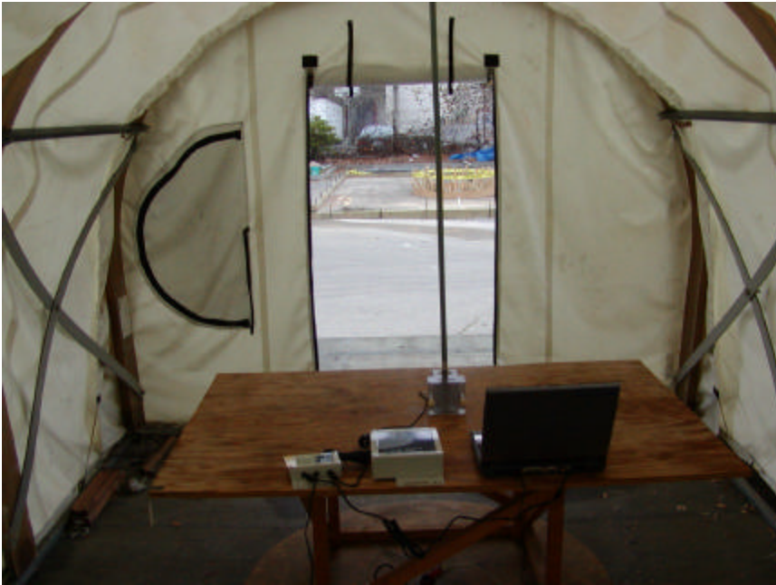
Radiated Emission – EUT with PAWOD24-12 12dBi Omni Directional Antenna Rear View
