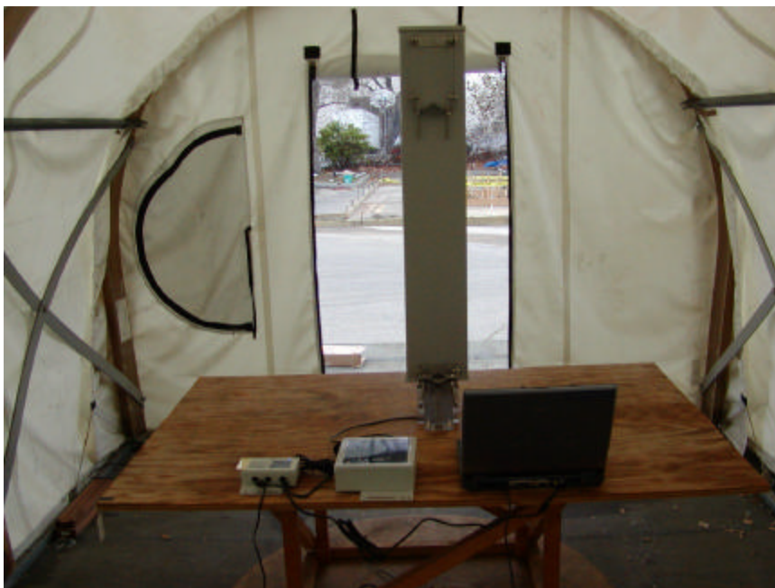
Radiated Emission – EUT with PAWSA24-16 16.5dBi Vertically Polarized 120 Degree Sector Antenna Rear View
