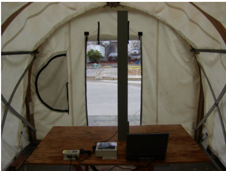
Radiated Emission – EUT with PAWSA24-16 16.5dBi Horizontally Polarized 90 Degree Sector Antenna Rear View
