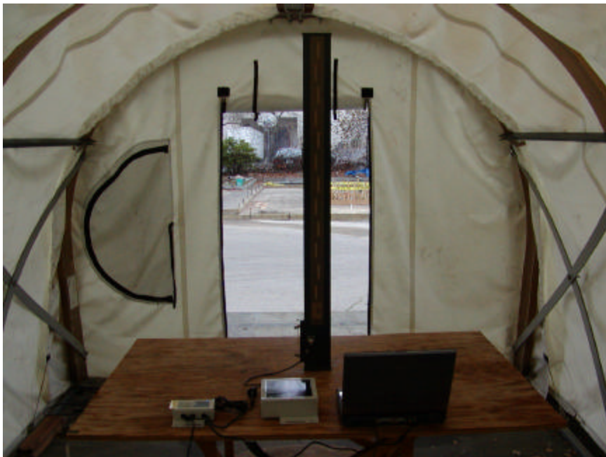
Radiated Emission – EUT with PAWODH24-13 13dBi Horizontally Polarized Sector Antenna Rear View
