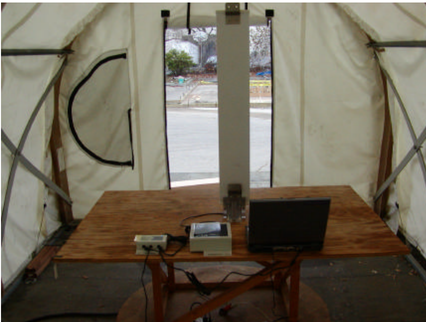
Radiated Emission – EUT with PAWSA24-17 17dBi Vertically Polarized 90 Degree Sector Antenna Rear View
