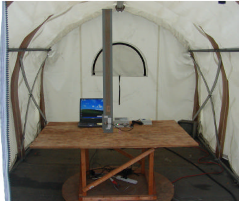
Radiated Emission – EUT with PAWSA24-16 16.5dBi Horizontally Polarized 90 Degree Sector Antenna Front View
