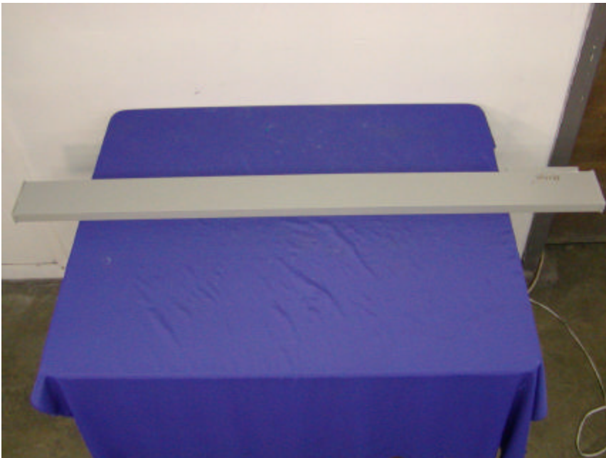
Antenna 5: PAWSA24-16 16.5dBi Horizontally Polarized 90 Degree Sector Antenna Bottom View
