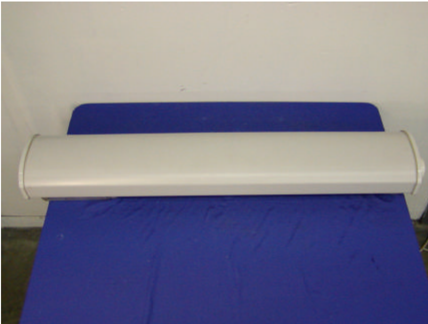
Antenna 9: PAWSA24-16 16.5dBi Vertically Polarized 120 Degree Sector Antenna Top View
