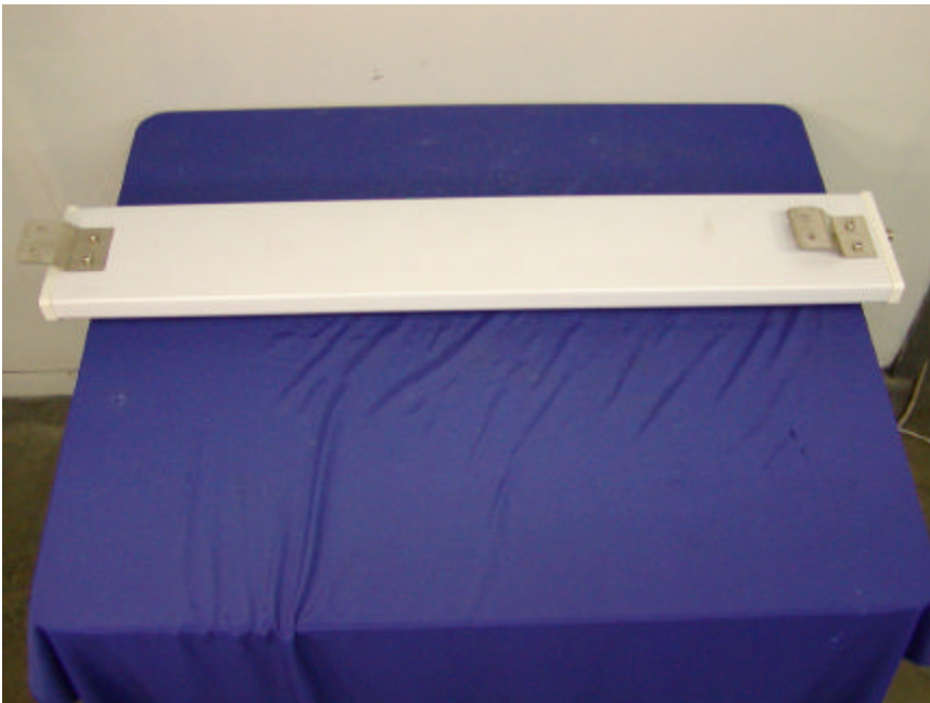
Antenna 8: PAWSA24-17 17dBi Vertically Polarized 90 Degree Sector Antenna Bottom View
