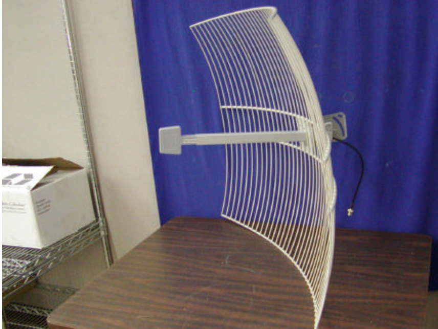
Antenna 3: WISP 24024 PTNF 24dBi parabolic Grid Rear View
