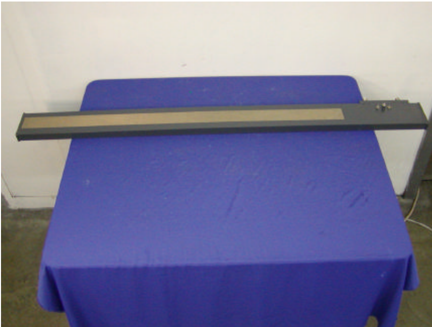
Antenna 7: PAWODH24-13 13dBi Horizontally Polarized Sector Antenna Bottom View
