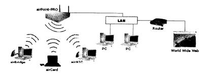
In this mode of operation, multiple wireless network Adapters can connect to an Access Point to form a complete Wireless network similar to a Wired LAN. Also, in this mode, the Access Point can act as a bridge between the Wireless and Wired LAN.
