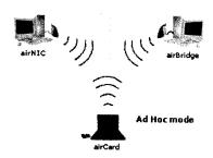
In this mode of operation, peer-to-peer (or point-to-point) connectivity is established between two PCs for Internet sharing, file sharing applications etc. Each PC is equipped with the Wireless client Adapter and they can talk to each other without an Access Point.
