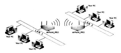
This mode lets one LAN talk to another LAN wirelessly linking two Ethernet LANs behind together. All the clients on both I ANs can talk to each other as if they are on the one bigger LAN.
