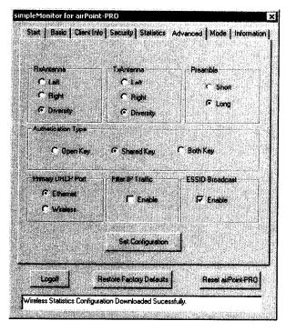
**RxAntenna**: Allows the user to select between Left and Right Antenna for Reception of signals. Diversity options will select the Antenna with best possible signal reception sensitivity(recommended).
