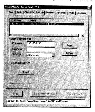
In case of a successful connection to the airPoint-PRO, simpleMonitor acknowledes by enabling all the tabs.
