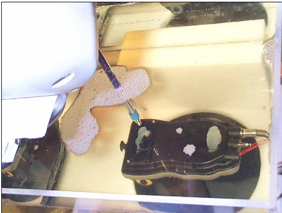
Figure 8. Positional photographs of SEMS Portable Unit with Positioned 1.5mm from Portable of Flat phantom see figure 3.
