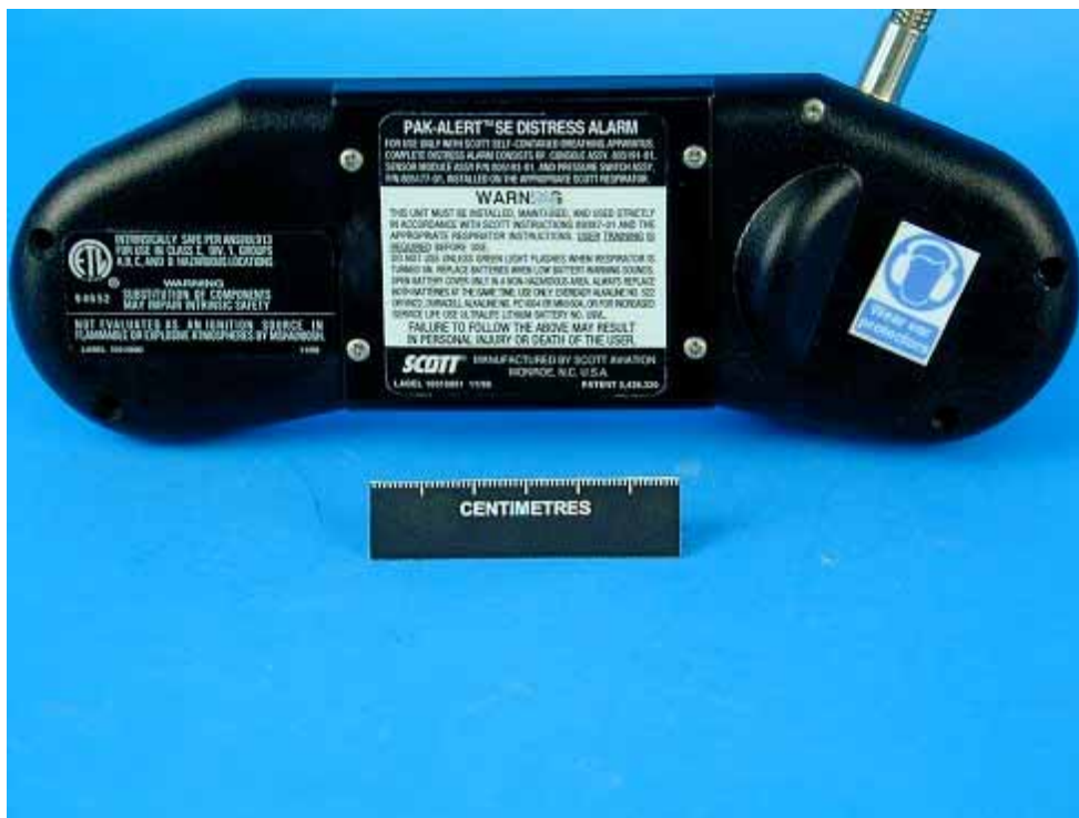
Figure 12. Closer view of SEMS Portable Unit Distress Alarm Unit.
