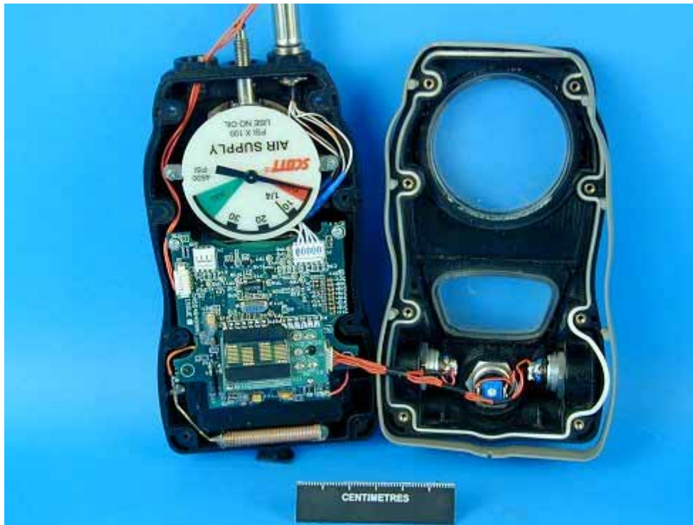
Figure 11. Internal view of the SEMS Portable Unit.
