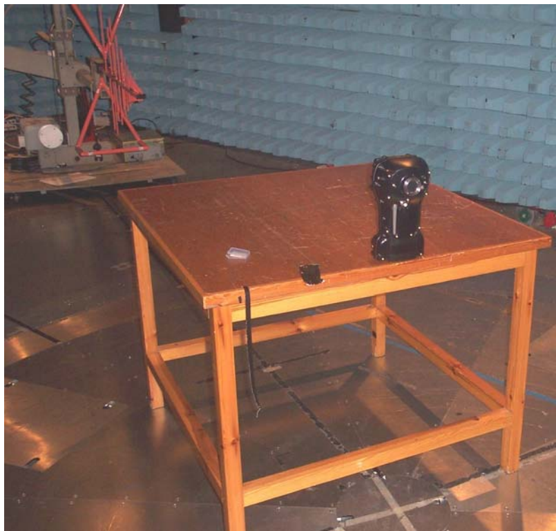
Photograph 1 Radiated Emissions Set Up
