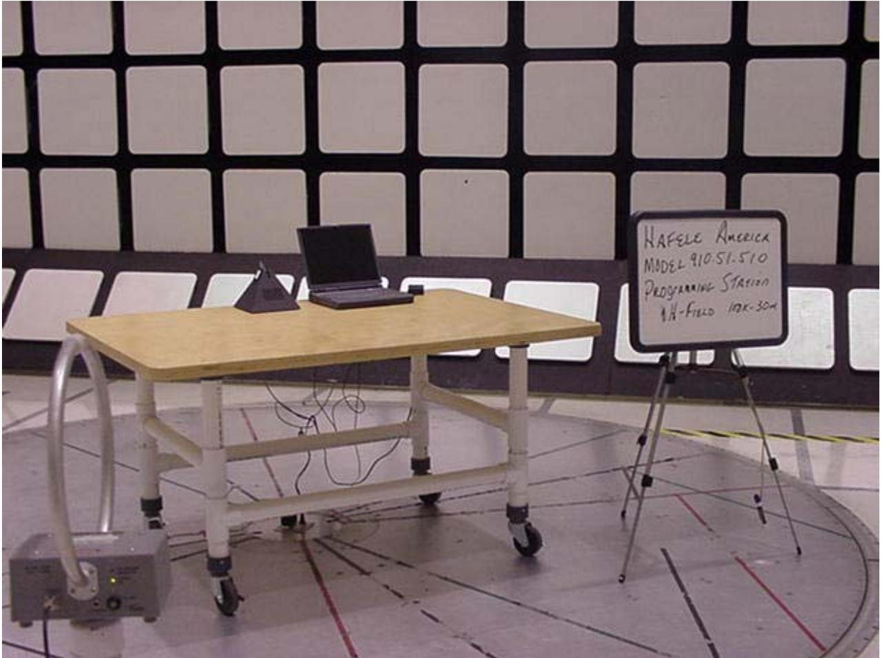
Radiated Emission Test .1 – 30MHz
