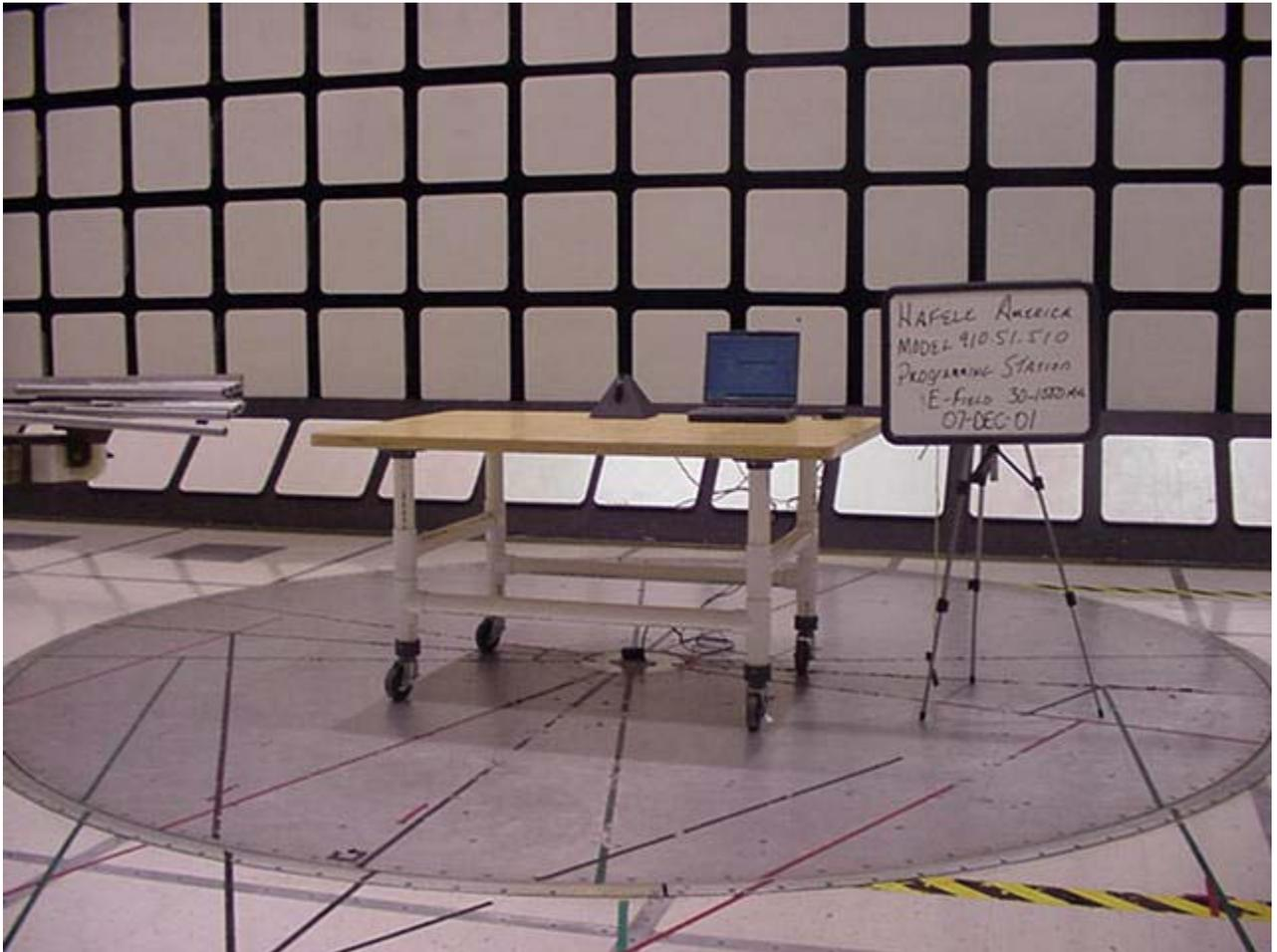
Radiated Emissions Test 30 – 1000MHz
