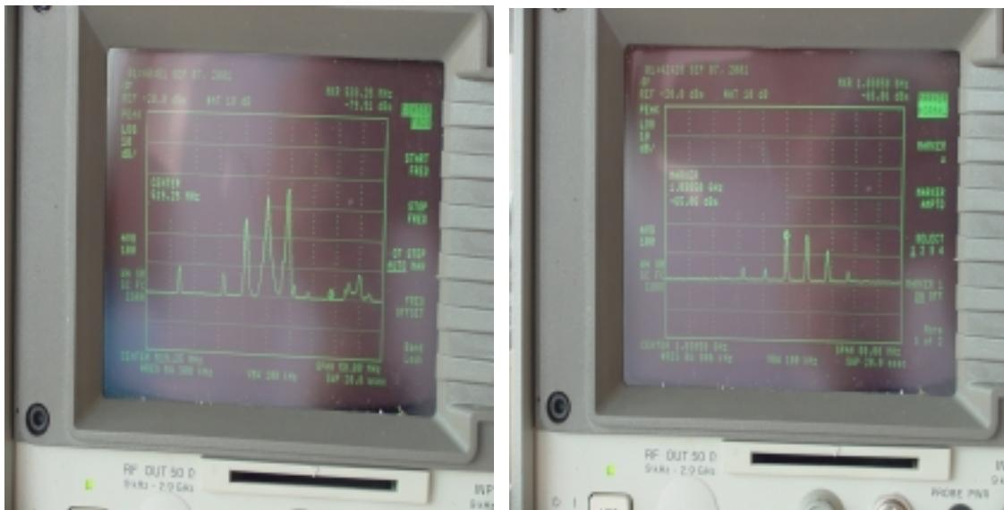
Worst case measurement of cabinet radiation measured just outside channel (left photo) and at 2<sup>nd</sup> harmonic area (right photo). Levels are tabulated below. All other levels were calculated below –80 dB relative to peak sync power and thus not tabulated.
