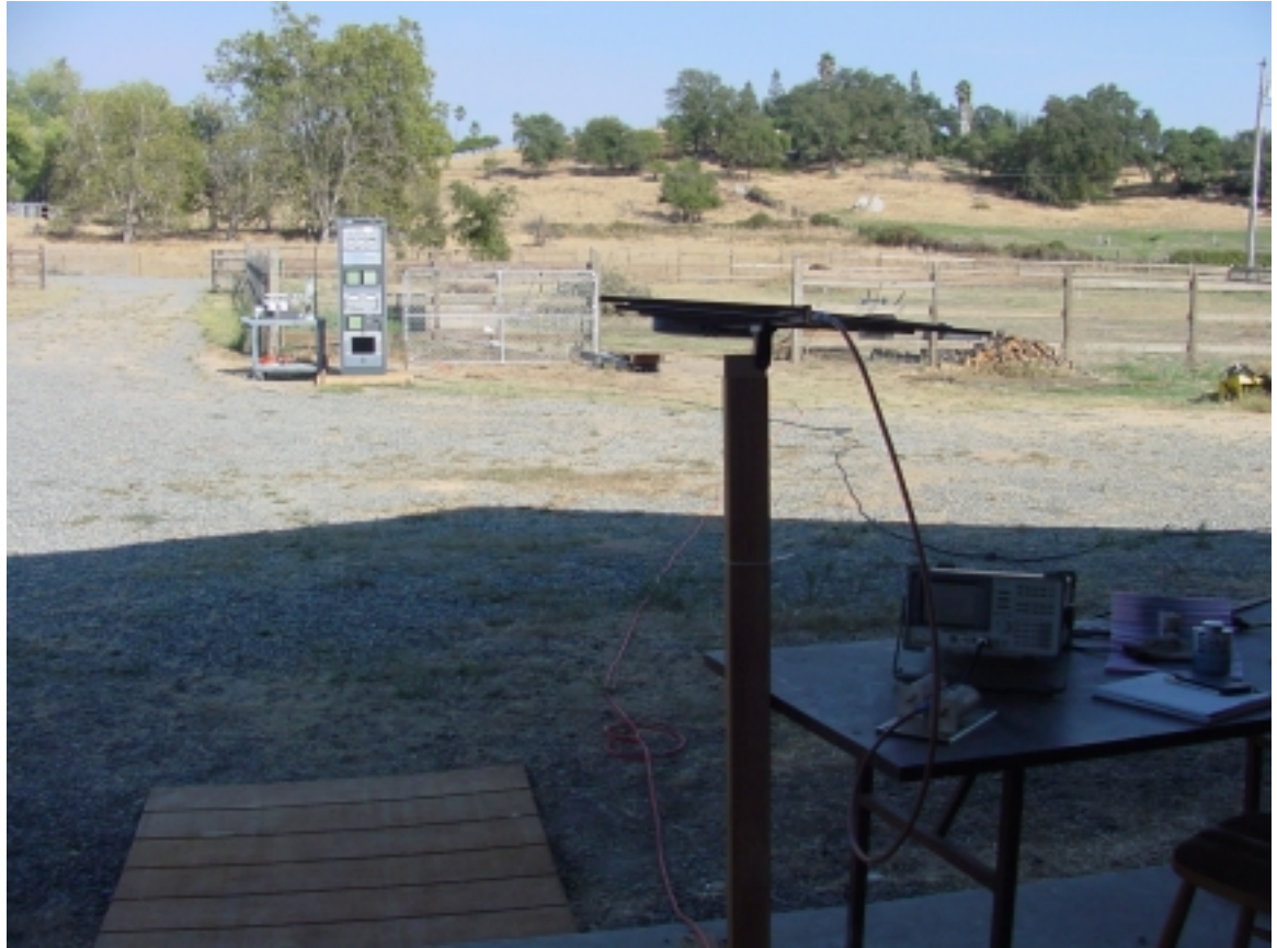
Figure showing Test setup for cabinet radiation. Cabinet was rotated to measure radiation from four angles. Foreground shows receiving antenna, notch filters, and spectrum analyzer.
