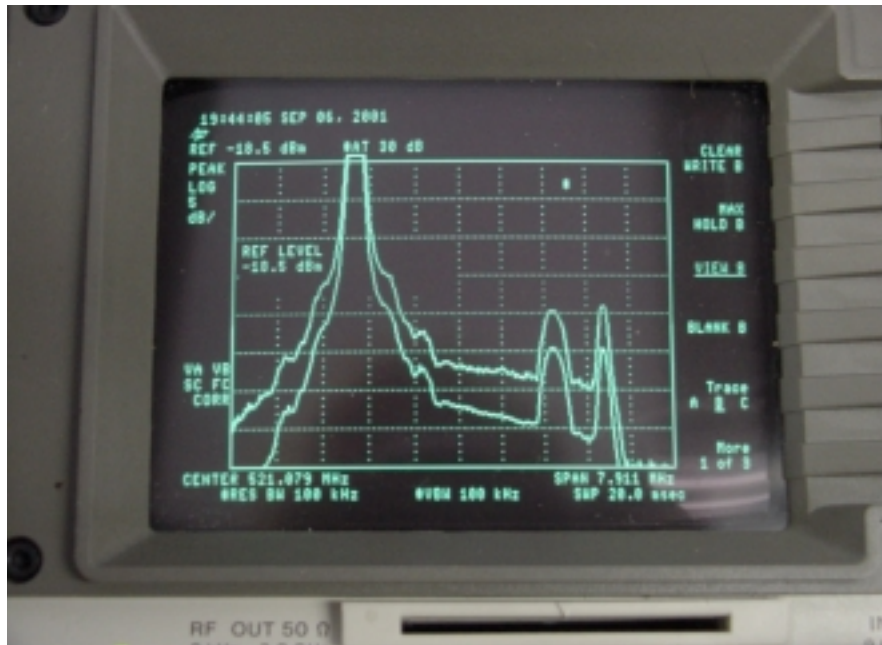
Output/ Input Frequency Response at 250 watts output (5 dB/div)
