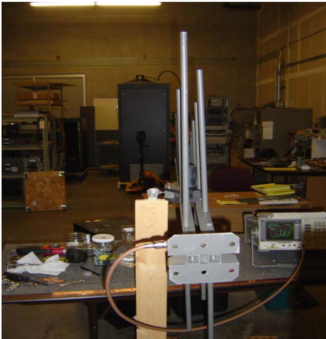
As indicated in the spreadsheet data on the following page, the worst case measurement was 62 dB at the second harmonic. (This photo on the next page shows this particular measurement). The measurement tables for all views of the transmitter at each frequency are shown below. The results indicate that all radiated harmonics meet the FCC requirement of 60 dB as outlined in FCC rule 2.1053 and 2.1057.
