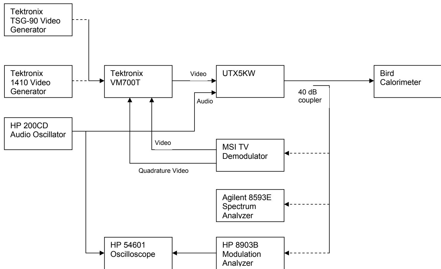
Dashed line indicates only one instrument connected at a time.
