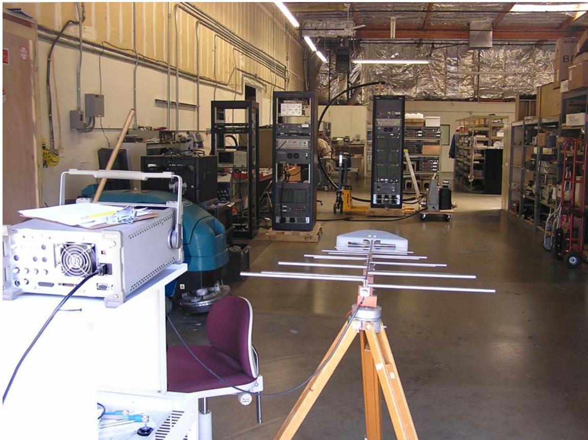
As calculated from the spreadsheet data on the following page, the worst case measurement was 66.8 dB at the second harmonic. (This photo shows this particular measurement). The measurement tables for the remaining views of the transmitter are shown below.
