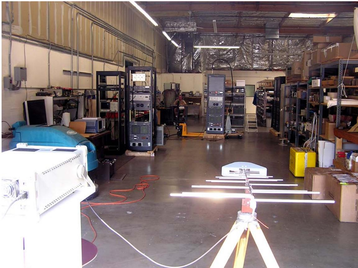
As calculated from the spreadsheet data on the following page, the worst case measurement was 65.1 dB at the second harmonic (The photo above shows this particular measurement). The measurement tables for the remaining views of the transmitter are shown on the following pages.
