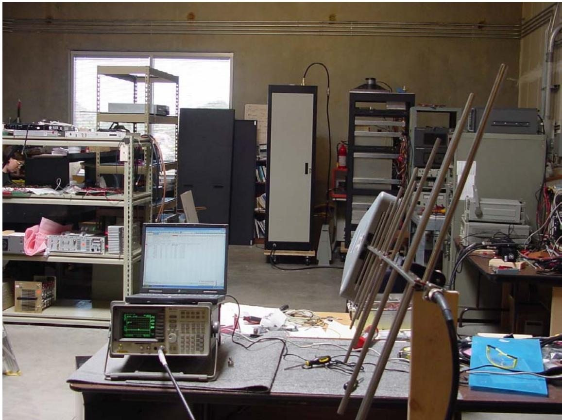
As indicated in the spreadsheet data on the following page, the worst case measurement was 83 dB at the second harmonic. The measurement tables for the remaining views of the transmitter are shown below. The noise floor of the measurement equipment was -88 dB referenced to the visual sync peak power and this level was recorded for frequency components that were less than or equal to -88 dB.
