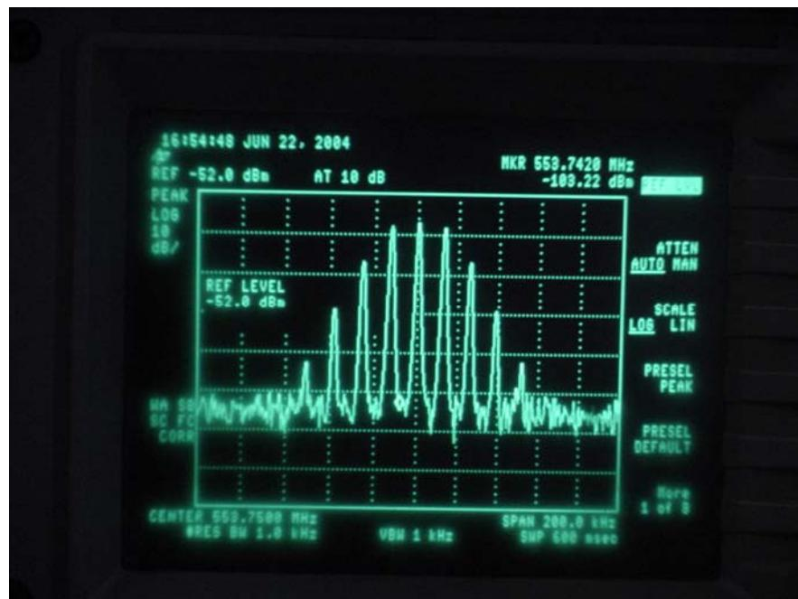
OCCUPIED BANDWIDTH—POWER OUTPUT = 100 Watts
