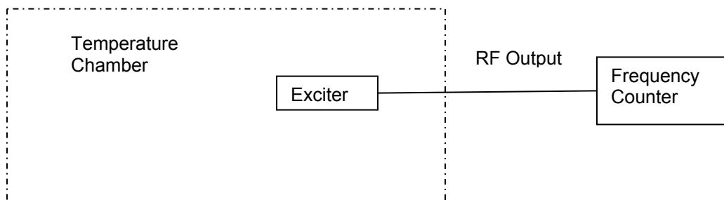
The variac was adjusted for nominal voltage and the frequency was recorded. Then the variac was adjusted to 85% and 115% of the nominal voltage and the frequency was recorded at each voltage level. The results are tabulated below.
