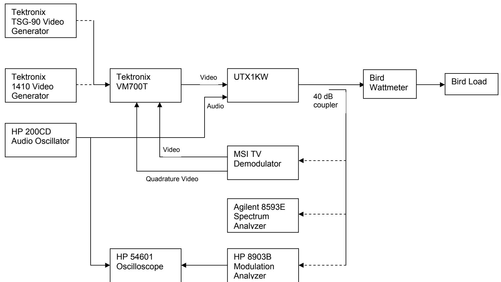
Dashed line indicates only one instrument connected at a time.
