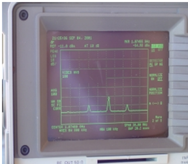
Worst case measurement of cabinet radiation measured at 2 nd harmonic of visual carrier.
