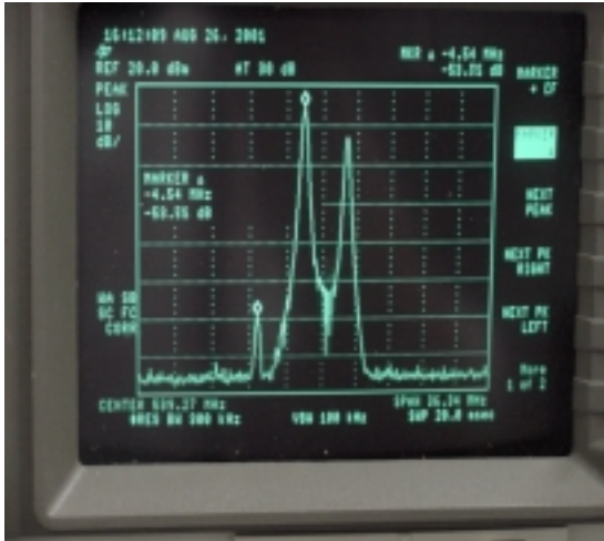
Adjacent channel spurious Output @ 110 watts peak
