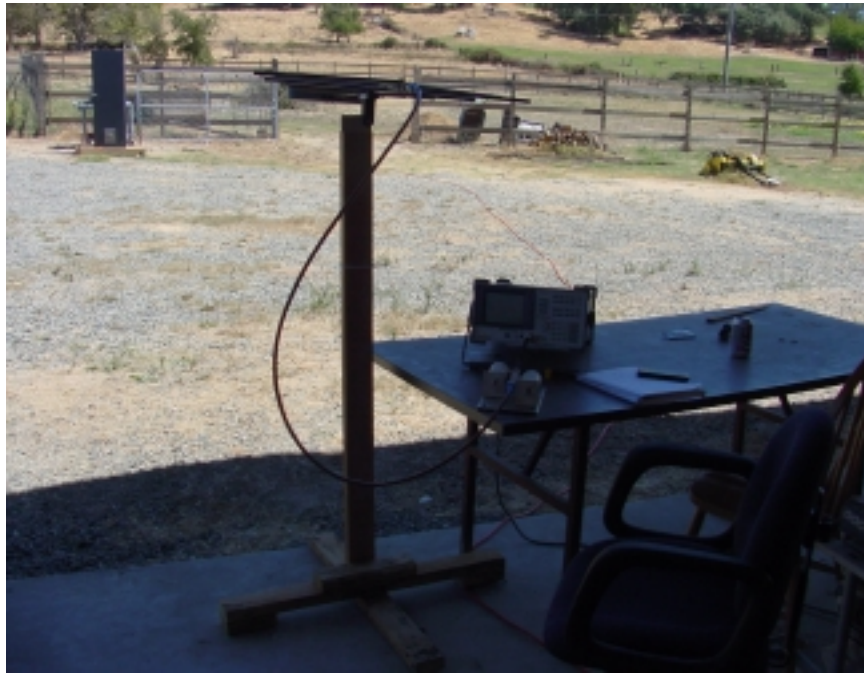
Figure showing Test setup for cabinet radiation. Cabinet was rotated to measure radiation from four angles. Foreground shows receiving antenna, notch filters, and spectrum analyzer.
