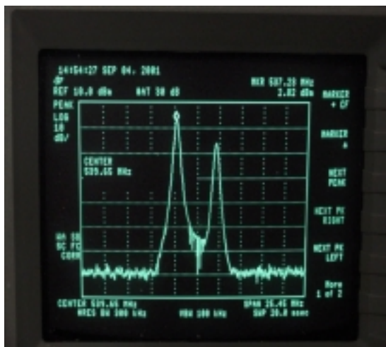
Adjacent channel spurious Output @ 30 watts peak
