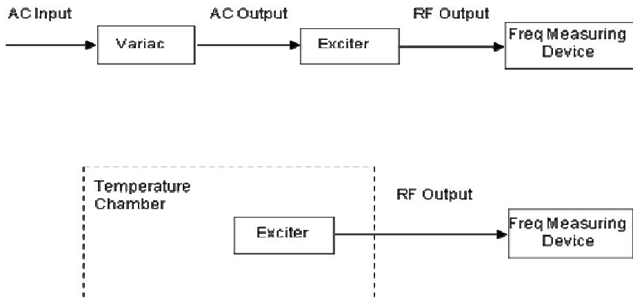
The variac was adjusted for nominal voltage and the frequency was recorded. Then the variac was adjusted to 85% and 115% of the nominal voltage and the frequency was recorded at each voltage level. The results are tabulated below:
