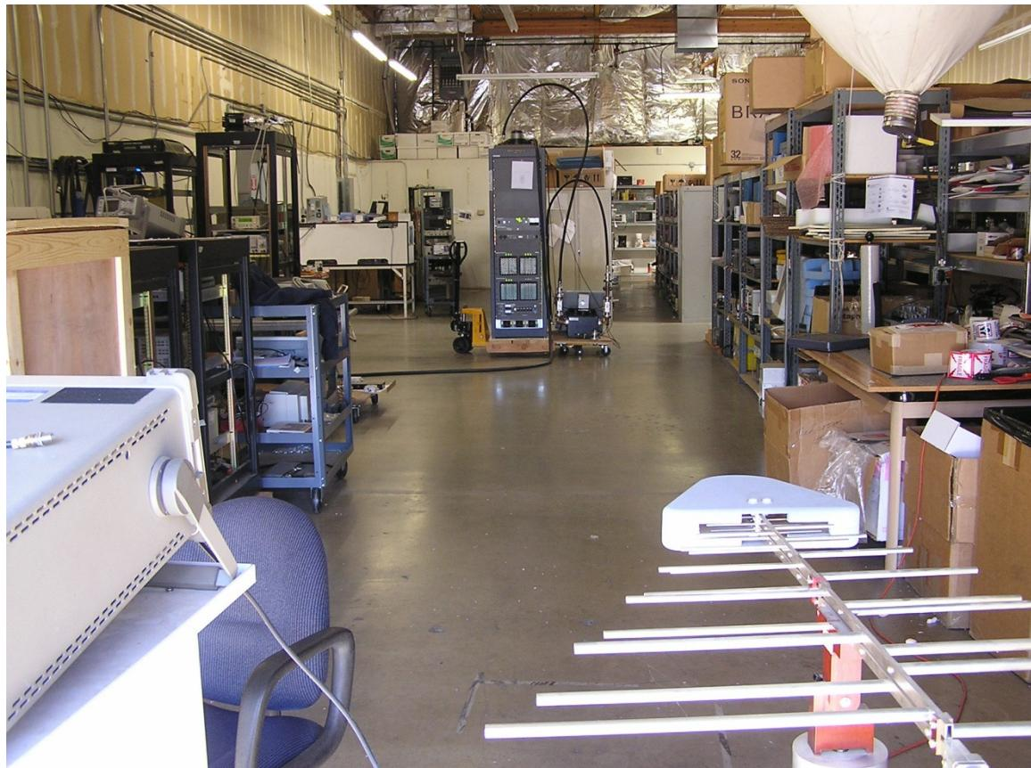
As calculated from the spreadsheet data on the following page, the worst case measurement was -70.2 dBm at the second harmonic. (The photo above shows this particular measurement). The measurement tables for the remaining views of the transmitter are shown on the following pages.
