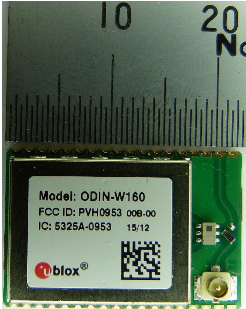
160912_4.jpg: EUT – Top View with shielding
